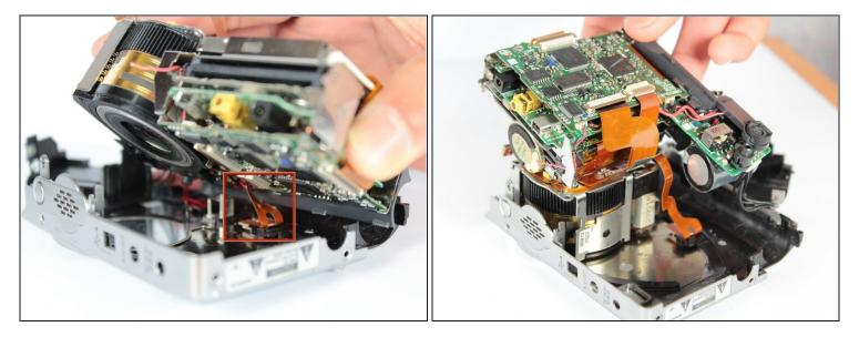
⚠ Do not fully separate the motherboard unit from the front cover. There is still a ribbon attached and it will rip.
