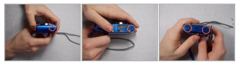
Remove four screws on the front case using a 00 Phillips head screwdriver. Two will be on the side with the camera strap, one on the bottom, and one on the side opposing the camera strap. They will be in pairs, one screw holding the front case and one screw holding the back case.
