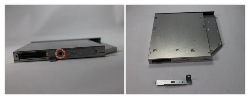
Face the side of the DVD drive that connects to the laptop and remove the 3mm screw with a Phillips head screwdriver.
