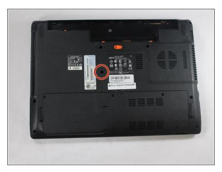
Remove the 7.0 mm screw, circled in the picture, using a Phillips head screwdriver.
