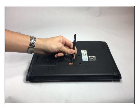
Use tweezers (or a similar tool) to slide the orange push pin. To release the battery, push it to the left.
