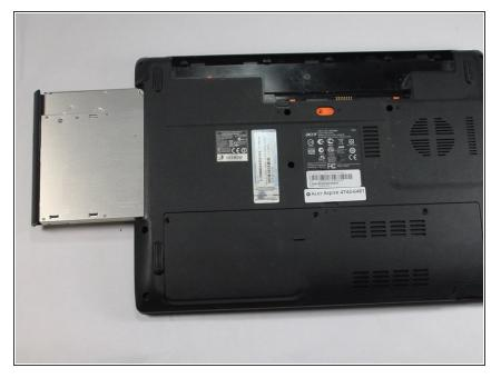
Once the screw is removed, the DVD drive should easily slide out
