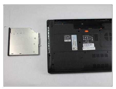
• Remove the drive completely.
