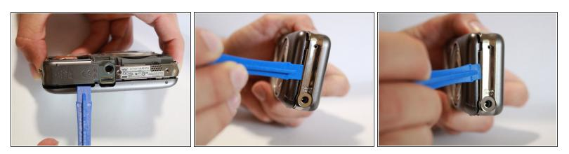
• Use a plastic opening tool to pry off the back casing.
