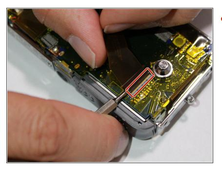
• Remove the LCD display by unplugging the connector.
