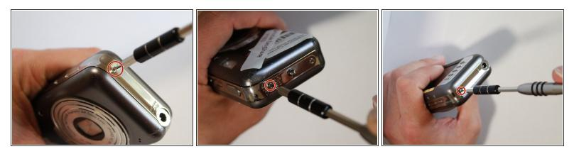
• Use a J00 screwdriver to remove the five exterior screws.
