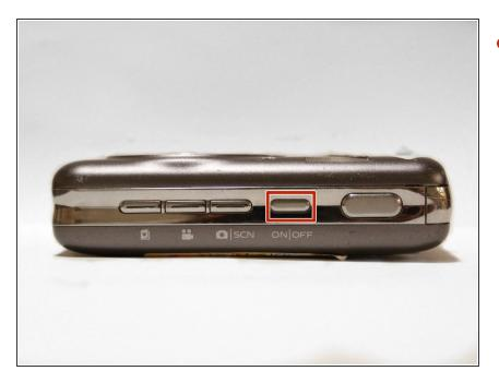
Turn off camera by firmly pressing the power button that is located on the top of the camera.
