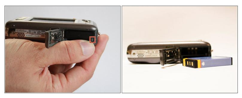
• Gently push the battery down until a click is heard. Battery should release and be lifted out of slot.
