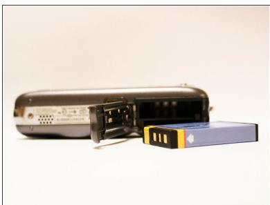
• Gently push the battery down until a click is heard. Battery should release and be lifted out of slot.
