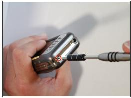
• Use a J00 screwdriver to remove the five exterior screws.
