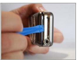
Use a plastic opening tool to pry off the back casing.
