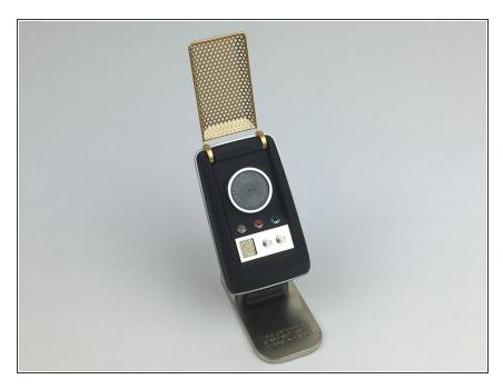
Power off the Star trek Bluetooth Communicator before disassembling by holding down the left button for five seconds. A "woosh-down" sound indicates the power is going off, and no lights will blink.
