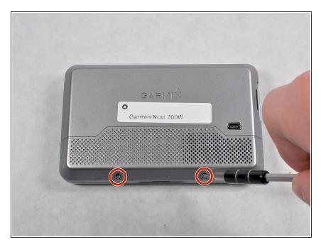
Remove the two 4mm T5 Torx screws.
