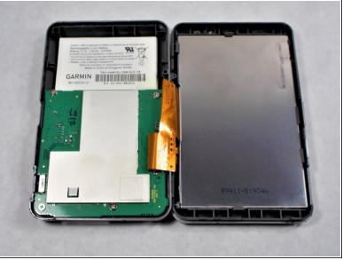
After the case front and rear are separated, carefully lay the two sides down without disconnecting or damaging the orange ribbon cable.
