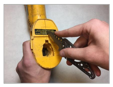
• Carefully cut the safety sticker with a blade along the seam.
