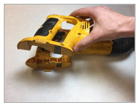
• Remove the Clam Shell from the handle unit.
