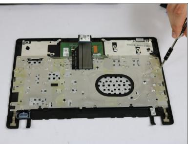
Using the JIS J1 Screwdriver Bit and Driver, remove the 17 screws (3.0 mm) from the back of the keyboard.
