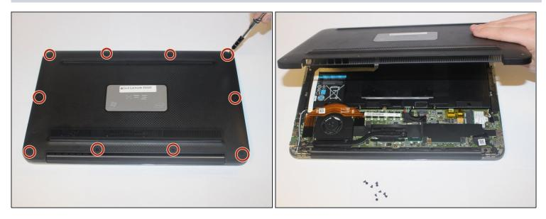
Remove ten 3mm screws from the back cover with a "T5" screwdriver.
