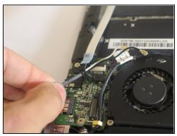
• After removing the battery, start to remove the wireless wire and making it through the other wires connected under the battery.
