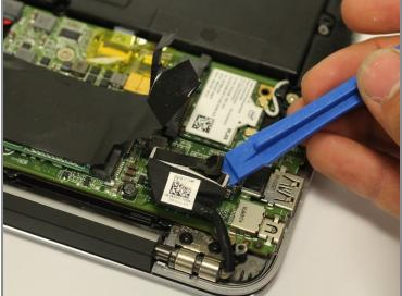
• Remove the black wire that connects the screen to the motherboard by pulling up with a plastic iFixit opening tool.
