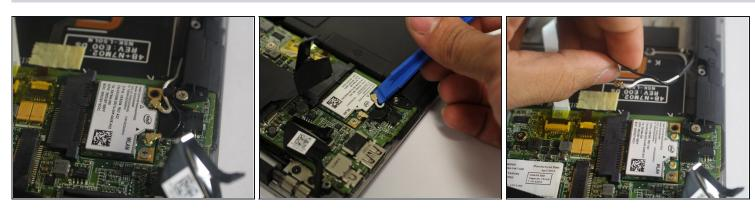
• Disconnect the wire that is connected to the wireless card with a plastic iFixit opening tool by lifting up slowly, then pulling the wires aside.
