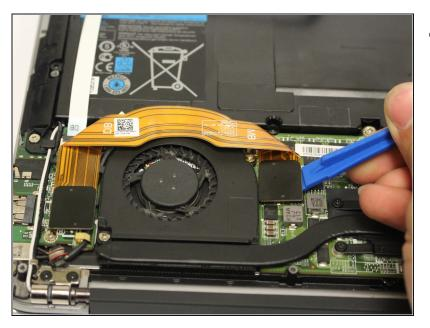
Remove the ribbons from both sides with a plastic iFixit opening tool.
