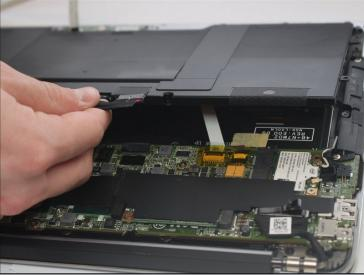
• Insert a plastic iFixit opening tool in between the port and the wires to remove the battery cable.
