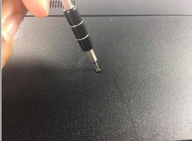
Locate and unscrew the screw which connects the optical drive to the chassis
