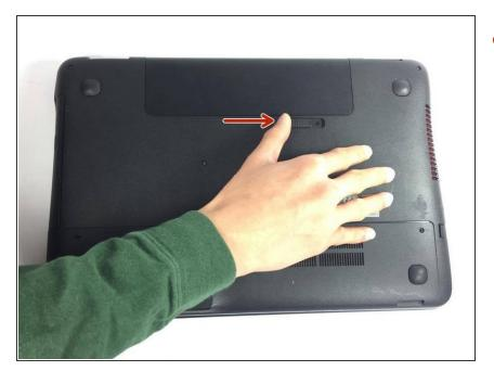
Push the latch found below the battery to the unlock position.
