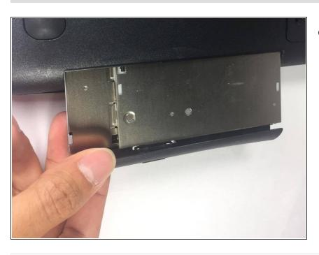
Pull on the optical drive gently. With little resistance, the optical drive should just slide out
