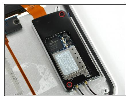
Remove the two Phillips screws securing the AirPort/Bluetooth bracket to the upper case.
