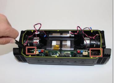
• Use tweezers to remove the two ribbon wires on the left and right side of motherboard.
