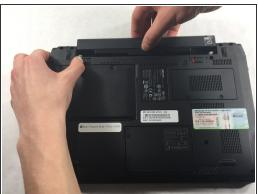
Unlock the right side of the battery by sliding the battery lock to the right. Then slide the left lock to the left and remove the battery.
