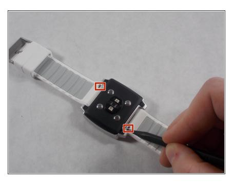
Release the spring latches on the underside of each band to remove the bands from the frame.
