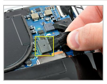
Disconnect the battery connector by pulling it straight out of its socket.
