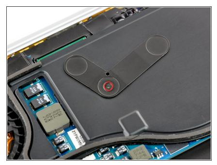
Remove the 1.9 mm Phillips screw securing the processor clamp to the heat sink.
