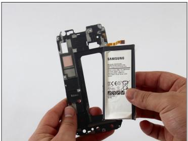
• Remove the battery from the frame.
