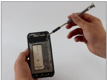
• Use the Phillips Head Screwdriver sized PH000 to remove the sixteen 4mm screws from the frame.
