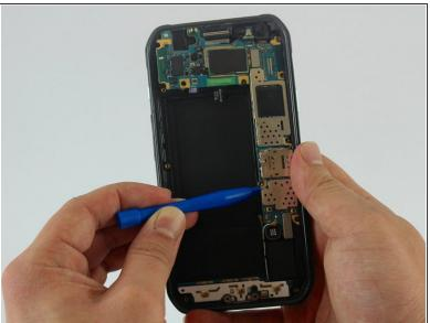
Insert the flats end of the spudger below the motherboard and twist it to pry the board up.
