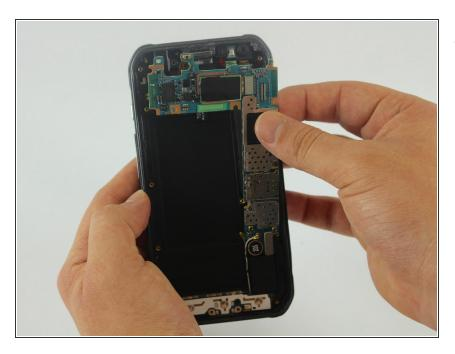
Remove the motherboard from the rear case.
