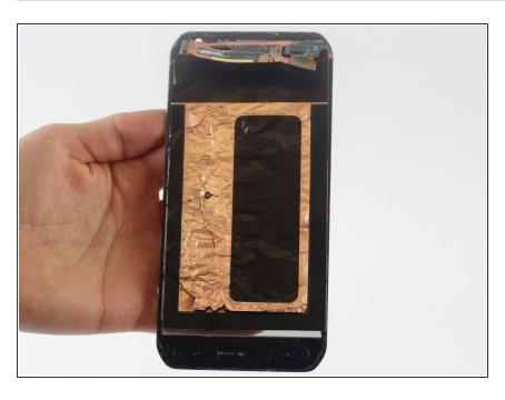
Remove the display assembly (LCD and Digitizer).
