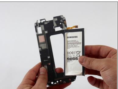
Remove the battery from the frame.
