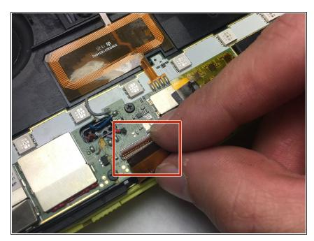
Remove ribbon cable from the circuit board.
