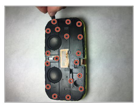
Unscrew eighteen 6.2 mm Phillips #0 screws and lift the black plastic plate from the case.
