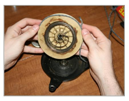
At this point add the new coil to the housing base. Snap the coil into position where the old on was.
