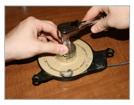
With this particular model there is a middle lock piece. Use a socket wrench to unscrew and release the coil.
