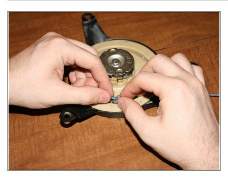
Untile the knot in the rope and slide it out of the housing.
