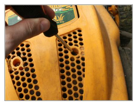
To begin the repair remove the protective casing. (This removal may vary with different lawnmowers.)
