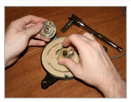
Once unscrewed, remove the metal piece which releases the tension on the coil.
