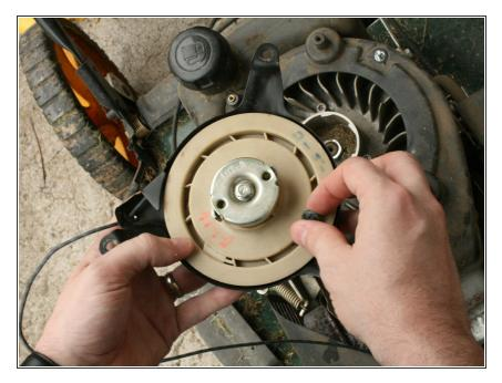
After removing the recoil, unscrew the cap that holds the pulley to the recoil starter housing.
