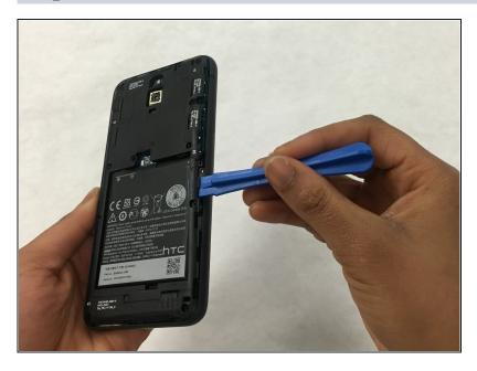
• Remove the black plastic circuit cover using a plastic opening tool.
