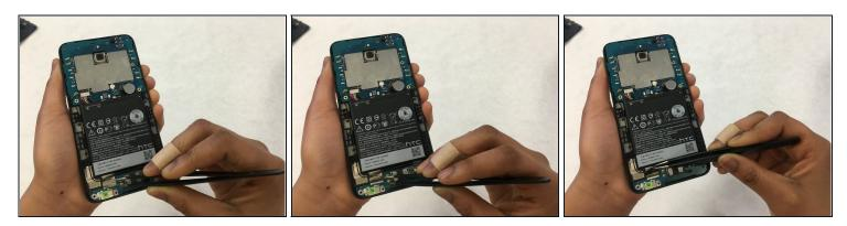
• Peel back the gray adhesive strip using the precision tweezers.
