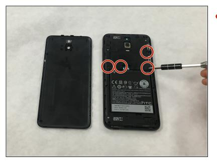
Remove the four black 4mm torx screws using the Torx T5 bit.
