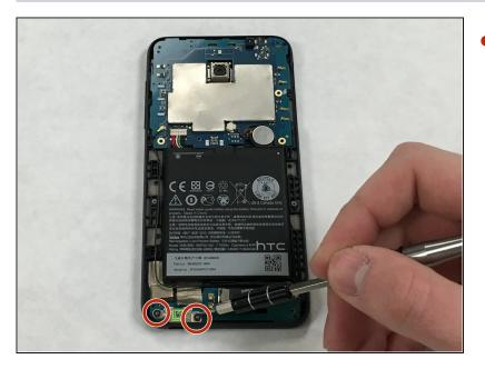
Remove the 4mm black Torx screw using a Torx T5 screwdriver.
