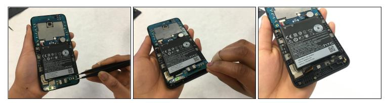
• Pry up the circuit board and pull it out using a pair of precision tweezers.
