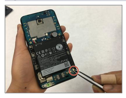
Using a pair of <u>tweezers</u>, disconnect the antenna wire.
