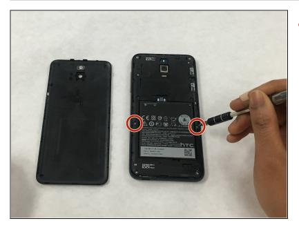
Remove the two 2.5mm phillips head screws using the Phillips 000 screwdriver.
