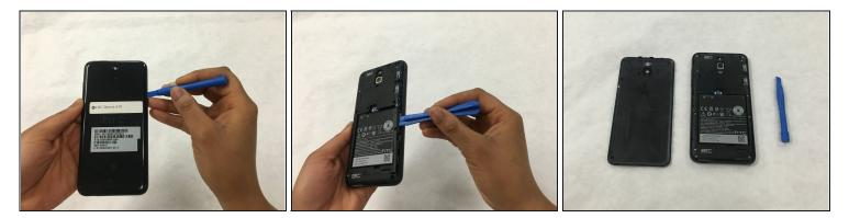
• Using a plastic opening tool, take off the back cover of the phone.
