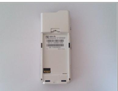
Remove the battery (which also functions as the back cover) from the device. This step is not
