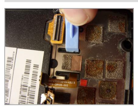
Using a plastic pry tool, lift and remove the three tabs securing the trackpad restrainer to the trackpad.
