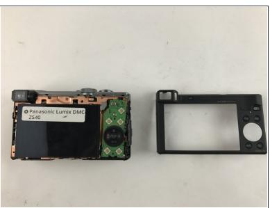
Pry off the back casing of the camera and place the camera face down.
