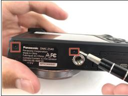
Unscrew the five 3mm screws located around the sides of the camera using a PH000 bit or Phillips 000 Screwdriver.
