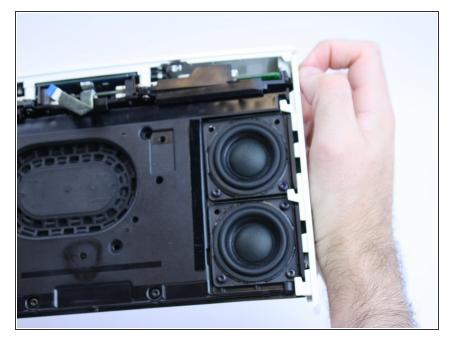
• With the bottom of the device facing you, pull down the trim pieces to remove from the device body.
