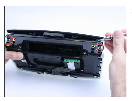
Remove the two screws using a torx screwdriver.
