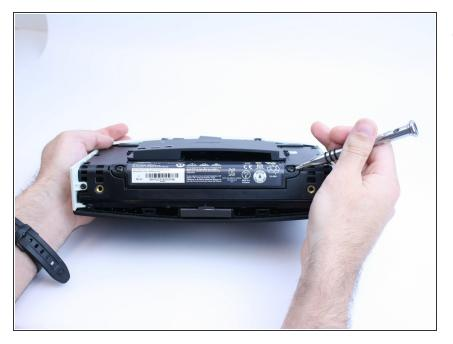
Remove the two T-10 machine screws, then pull the battery straight out.
