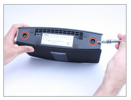
Remove the two T-10 machine screws at the bottom of the device.
