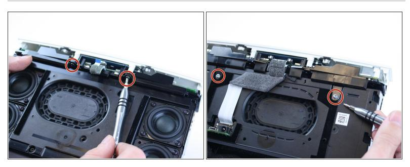
Remove four T-10 Torx screws; there are two on the front and two on the back.
