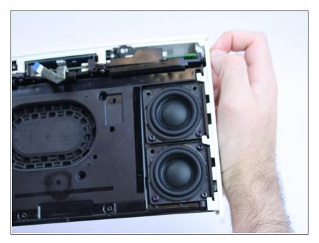
With the bottom of the device facing you, pull down the trim pieces to remove from the device body.
