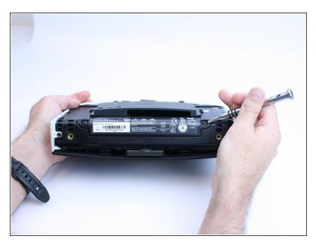
Remove the two T-10 machine screws, then pull the battery straight out.
