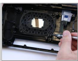
• Remove the four screws from the subwoofer and lift it out of the casing.
