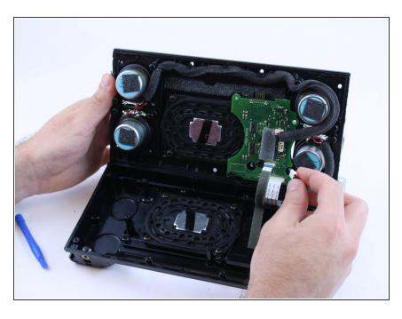
Gently pull on the connectors at the circuit board to remove. Remove the screws from the circuit board and set the board aside.
