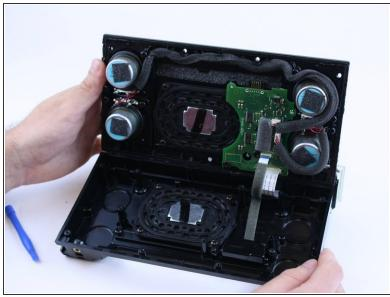
Separate the case that holds the subwoofer in place.
