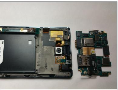
Using a spudger or small prying tool, lift up the motherboard from the chassis of the device.
