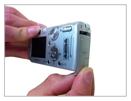
• Pull the battery cover in the direction of the arrow.
