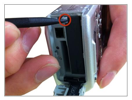
Push the battery latch away from the battery until the battery is released. Then remove battery.
