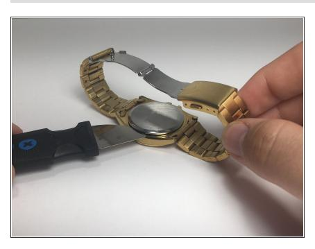
Locate the notch under the back cap of the watch. Wedge the jimmy into the notch, and pry off the back.
