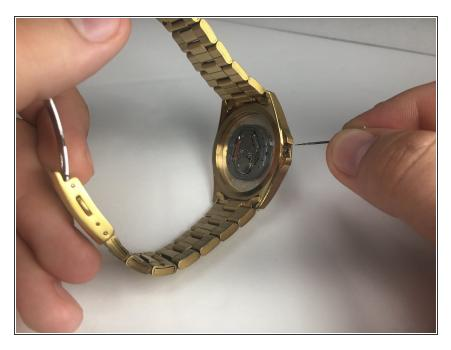
Insert the crown stalk into the crown stalk holes.
