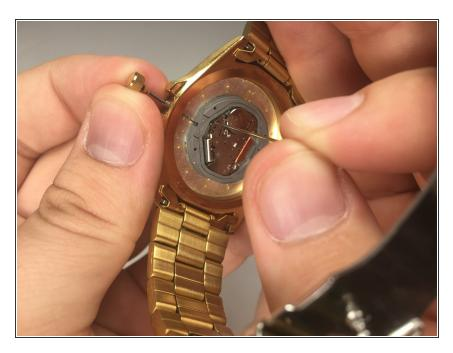
Remove the crown stalk by placing the needle in the release notch. This will release stalk and allow it to slide out.
