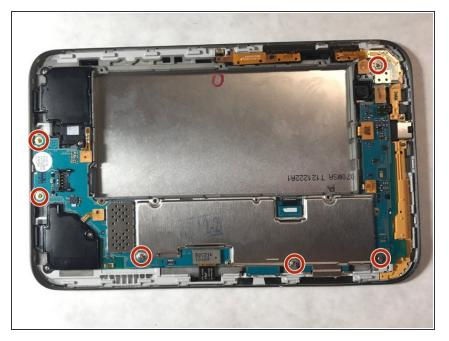
Using a phillips head screwdriver, remove the 6 4mm screws holding the motherboard in the device.
