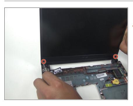
Unscrew the two 4mm phillips head #00 screws.
