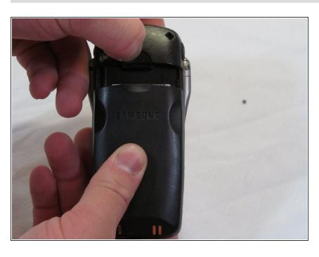
Slide the battery toward bottom of the phone, about a quarter of an inch, to clear the hooks that keep it secured to the back of the phone.
