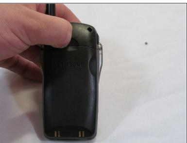
Place the phone so that the back is facing you. Depress the locking tab on the back of the phone with a finger or thumb.
