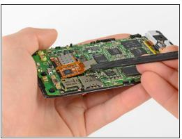
Use the flat end of a spudger to pry the three display cable connectors off their sockets on the motherboard.
