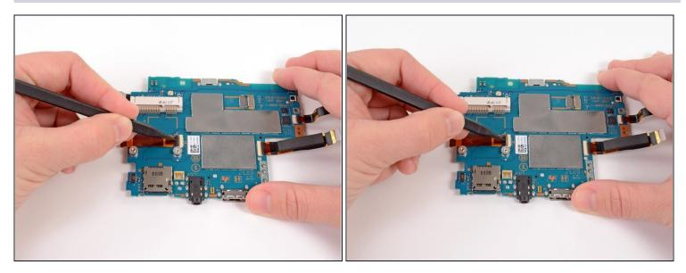
• Using a spudger, release the tab on the ZIF connector located above the two screw posts where the wireless card once was.
