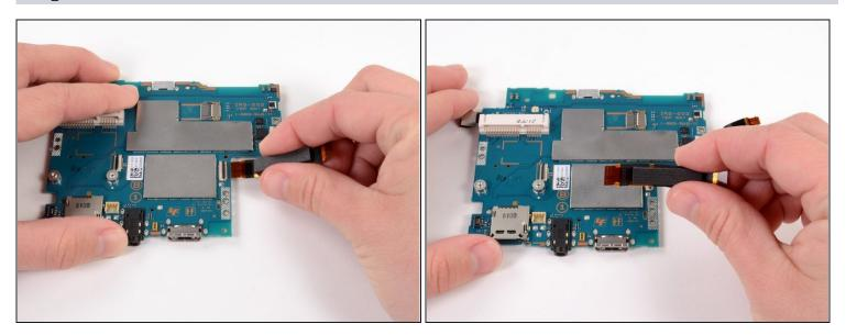
• Gently pull the flex cable out of the ZIF connector, and remove it.
