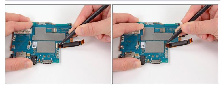
• Release the tab on the large ZIF connector on the right side of the motherboard by lifting the tab with a spudger.
