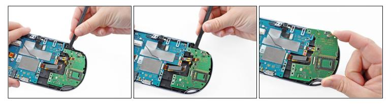
• Starting from the upper left corner, use a spudger to pry up and remove the left button board.
