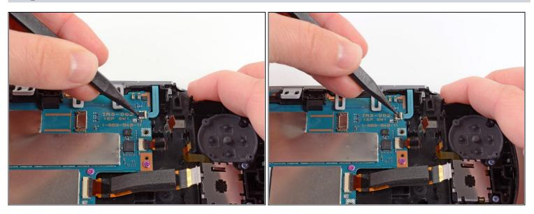
• With the help of a spudger, lift and release the tab on the blue flex cable socket.
