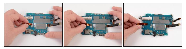
• Gently pull the flex cable out of the ZIF connector, and remove it.
