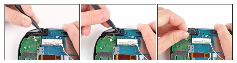
• Pry up the right shoulder button casing with a spudger and set it aside.
