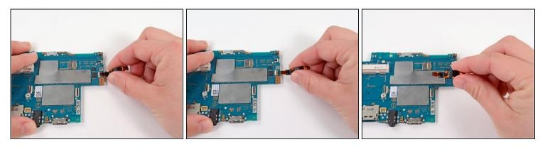
• Gently pull the flex cable out of the small ZIF connector, and remove it.
