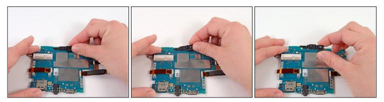
• Starting at the right side, gently lift and remove the black casing that once held the camera.
