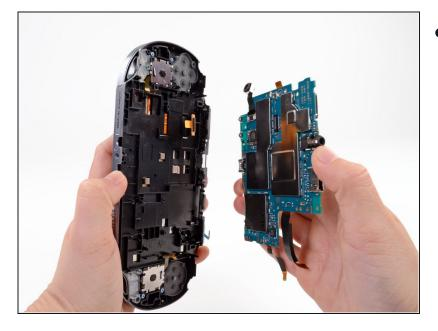
• Completely separate the motherboard from the case. Remove the case.
