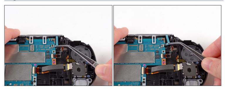
• Using <u>tweezers</u>, gently pull the blue power flex cable out of the socket; rest it out of the way.
