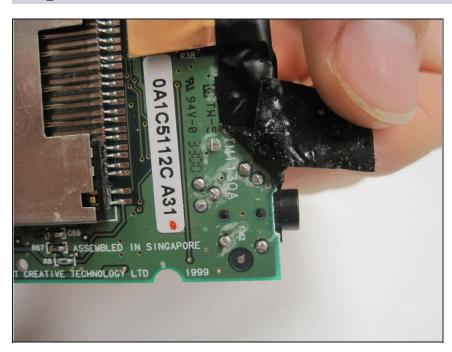
Gently remove the black adhesive tape from the underside of the headphone jack.
