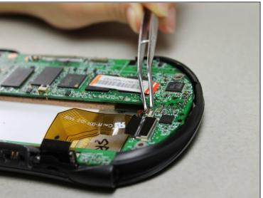
• Disconnect 2 brown wire-tape ends from each end of the motherboard. Gently pull straight out with tweezers.
