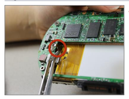
Disconnect the 2 brown wiretape ends from the left side of the battery slot on the motherboard using tweezers.
