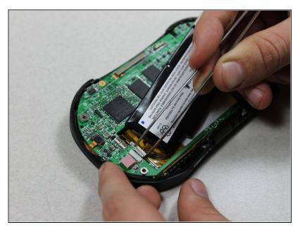
Slowly pull the white plug from its receptor. Grasp its sides firmly with a pair of tweezers and gently wiggle from side to side.
