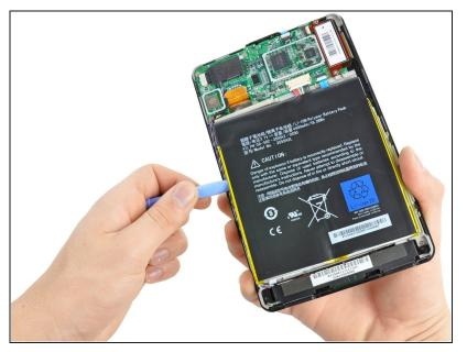
Repeat the process from the previous step to free the left battery cell.
