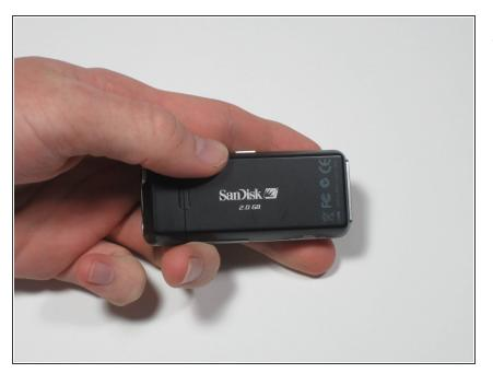
Slide the back cover forward toward the top of the device with your thumb.
