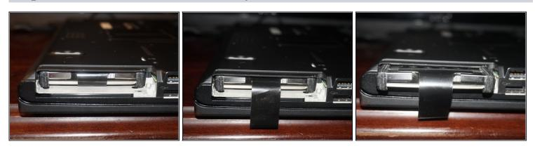
Pull the black tab on the drive caddy to remove the drive.
