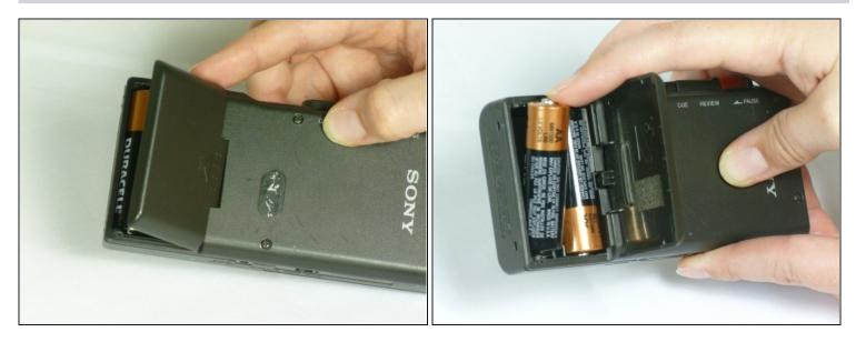
• Lift the cover and remove the batteries.
