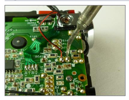
• Desolder the two connections between the wires and the motherboard. Make sure that the two solder points do not melt together.
