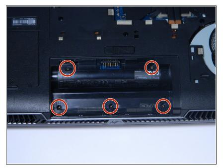
Remove the 5 screws circled in the picture, located where the battery pack once was.
