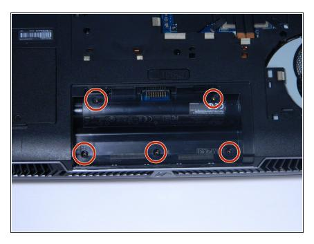
Remove the 5 screws circled in the picture, located where the battery pack once was.
