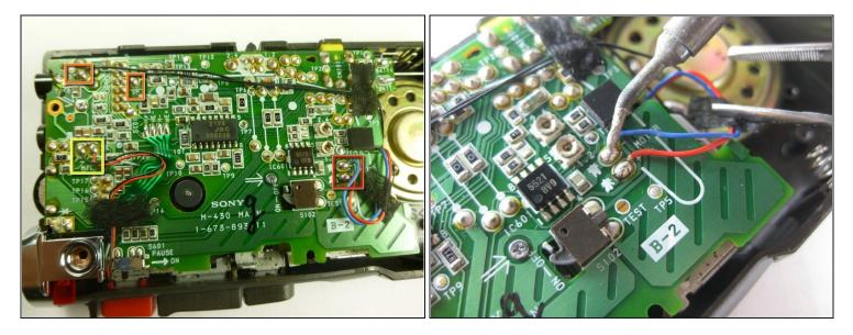
• Desolder all wires connecting components to the motherboard.
