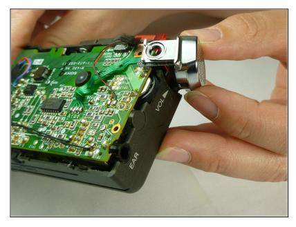
• After desoldering the microphone connections, pull the microphone straight out from the device and set aside.
