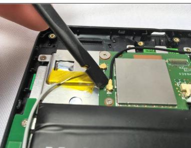
Remove the 5 antenna cable connectors from the motherboard using a spudger.
