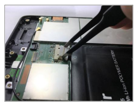
Use the tweezers to carefully disconnect the power cable bundle from the motherboard.
