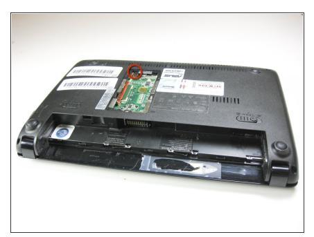
Remove the single 6.65 mm screw next to the RAM socket.
