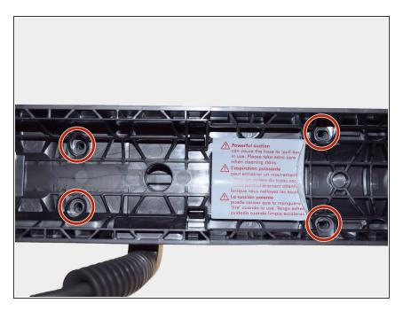
Remove the four 15 mm T-10 black screws now showing in the back of the vacuum hose track, using the Phillips 0 screwdriver found in the iFixit tool kit.
