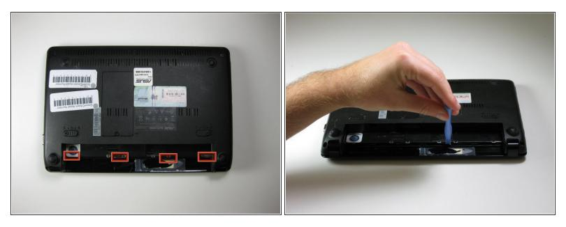
• Use a plastic opening tool to pull up the four metal latches in the battery cavity that is located on the bottom of the laptop.
