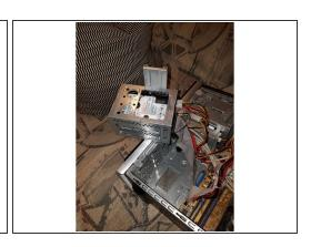
Once you've done that then push the button down closer to the logic board right next to it the HDD deck and slide it to the right and pop it out.
