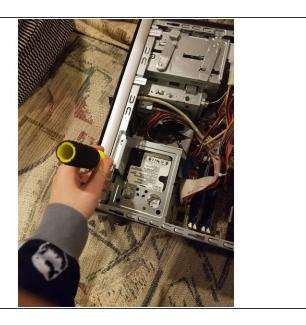
After you do that then unscrew the two Phillips types screws holding in the HDD deck by the front panel.
