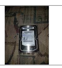
Unscrew the four screws holding the HDD in then take that unplug it and then take it out of the deck.
