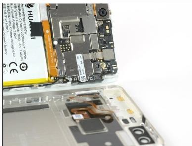
Disconnect the fingerprint sensor using a spudger.
