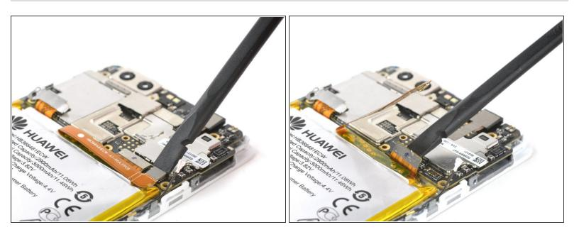
... as well as the battery connector and the cable running to the daughter board.
